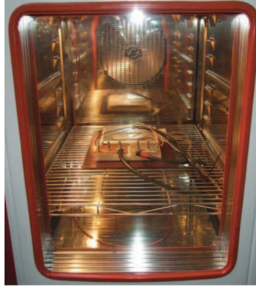
Figure 14: Test cell at constant temperature in a climate chamber.
