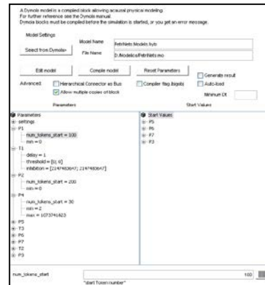
Figure 11: Parameter dialog of the DymolaBlock in Simulink
